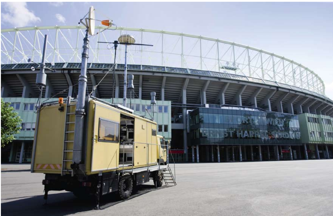
FIG 1 Test vehicles positioned in the vicinity of stadiums in spots especially suitable for conducting radio measurements were integrated into the DF and monitoring network (here outside the Ernst Happel Stadium in Vienna).
