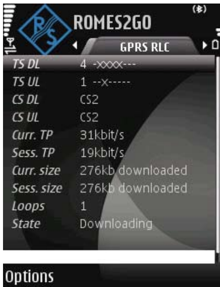
FIG 5 Number of timeslots used and the coding scheme of (E)GPRS.
