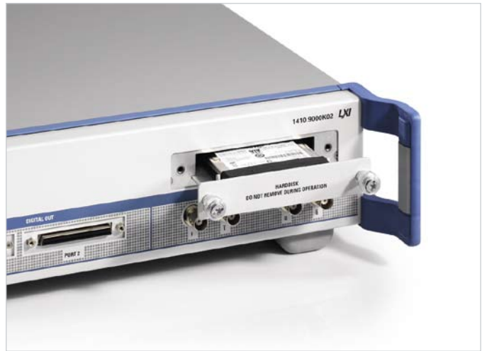
FIG 5 The removable hard disk is a must for military applications so that confidential data remains in a secured area when the generator is being serviced.
