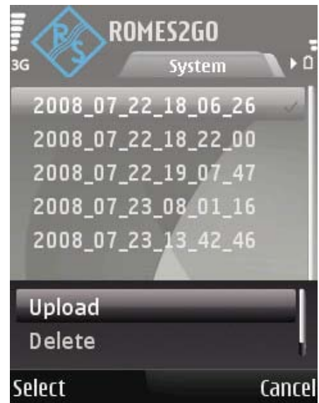
FIG 7 Transfer of the measurement file to a server via FTP.
