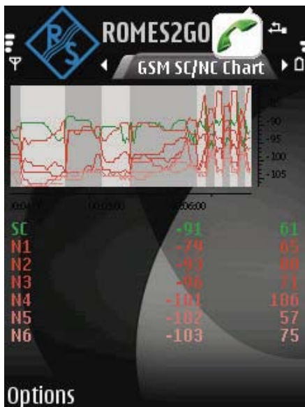
FIG 2 Graphical/numeric display of the GSM measurement report.
